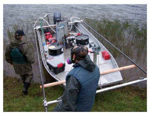
Figure 11. Motorboat and a well-pipe boom system currently used by the Alaska Department of Fish & Game for deep-water application of rotenone. It may be used if Sonar Genesis is applied in mid- to late-summer when thermoclines may develop in Beck and Daniels Lakes.
