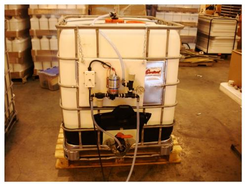
Figure 10. 12-volt electric pump system with 30-50 gallon tank will be used with PVC boom to apply Sonar Genesis below the water surface.
