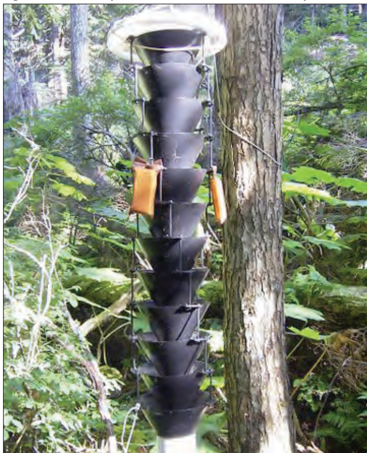
Figure 8. Funnel trap used to monitor for exotic insect pests
