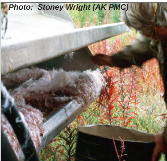
Figure 23: Collected fireweed stays in the seed stripper until removed for processing
