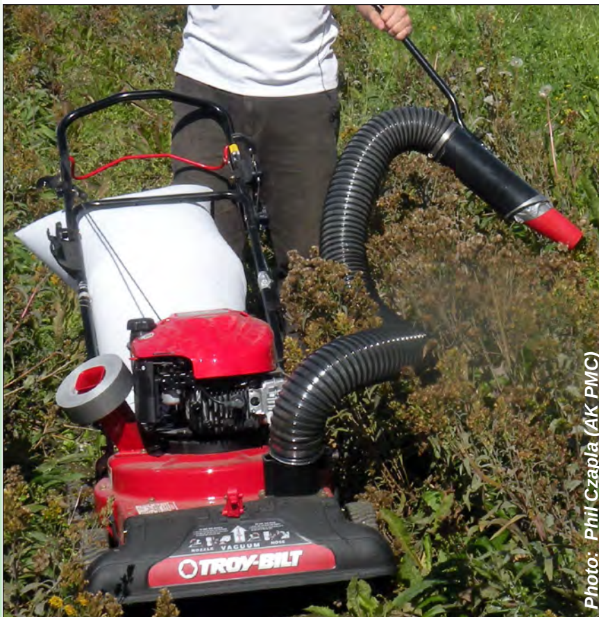
Figure 26: A chipper shredder with a vacuum used to harvest seeds
