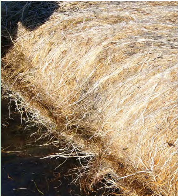
Underside of vegetation mat, showing developed roots intertwined with erosion control fabric
