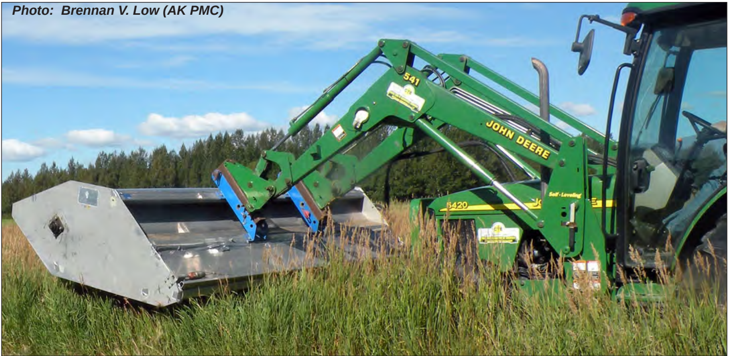
Figure 25: Using a seed stripper leaves the inflorescence (seed-head) intact, allowing for multiple equipment passes
