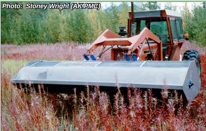
Figure 22: A Woodward Flail-Vac © seed stripper attachment is used to collect large amounts of wild seed, such as fireweed
