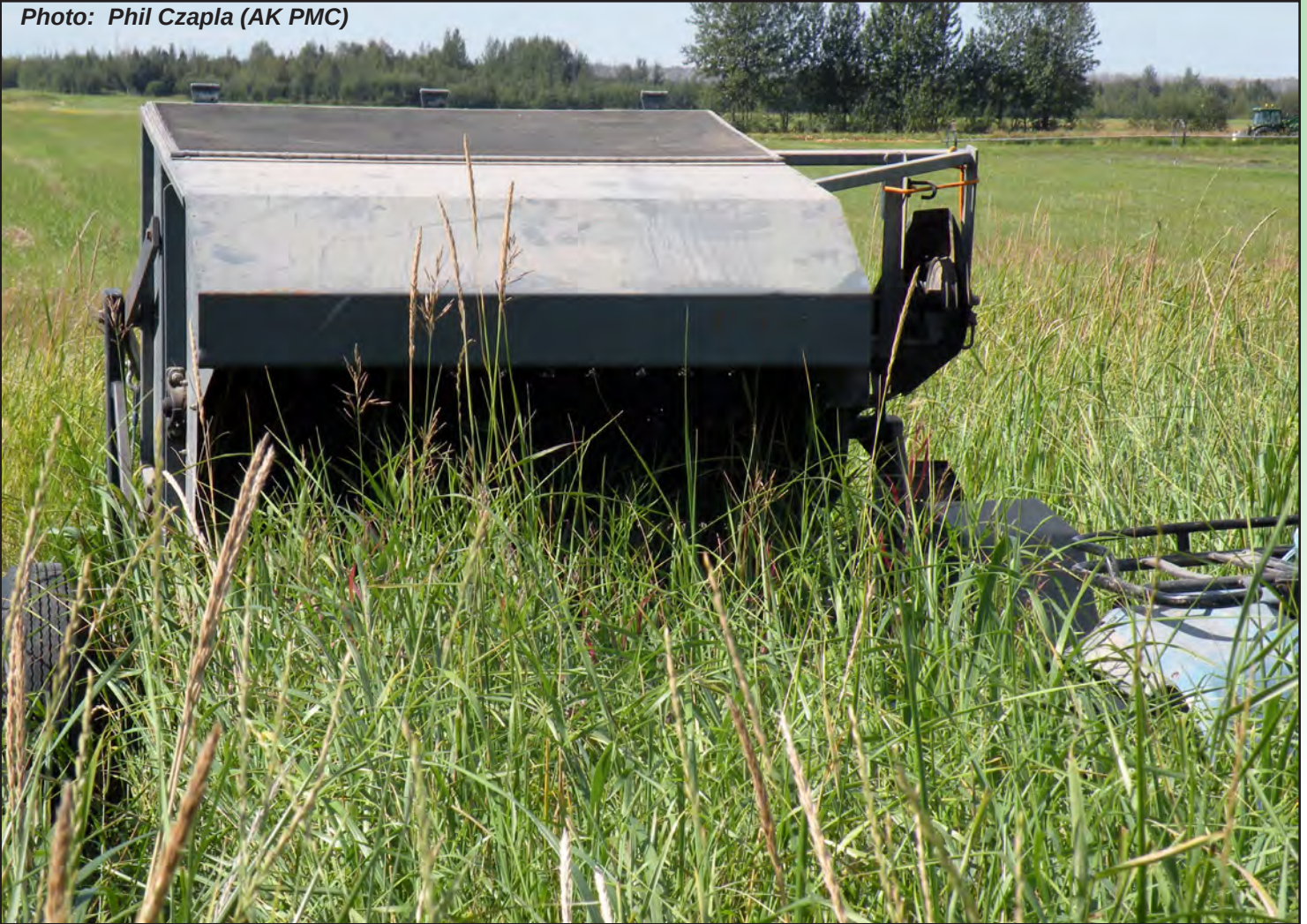
A pull-type seed stripper is an effective means of harvesting collections of wild seed
