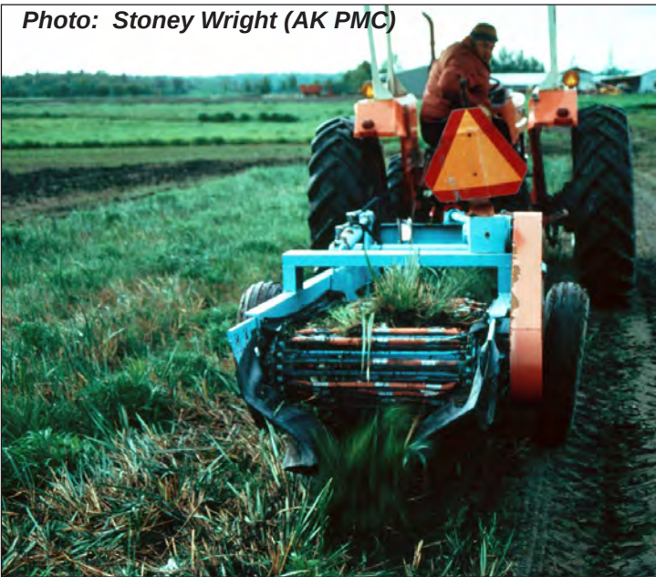
Figure 20: A tractor mounted potato harvester being used to harvest Beach Wildrye
