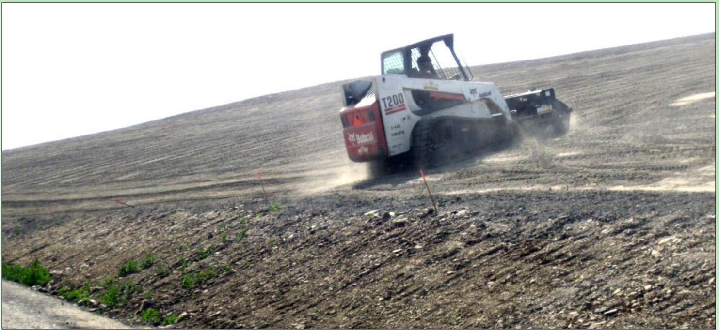
A Bobcat T-200 dozer with a drill seeder attachment applies a seeding mixture to the site.
