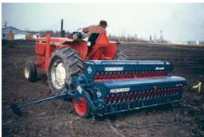
Figure 85: Drill seeders are specialized types of equipment that work best on level sites with fine soils.
