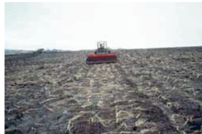
Figure 86: Brillion seeders are forgiving and can be used on gravelly and rocky sites more reliably than other drill seeders.
