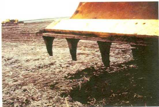
Figure 3.7.9 "Tiger Teeth" on Dozer Blade.
