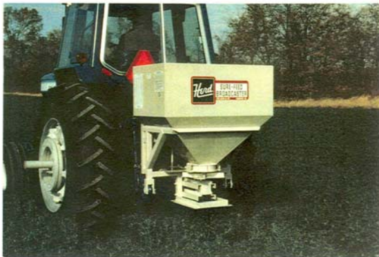
Figure 3.5.3 Spinner Type, PTO Driven
