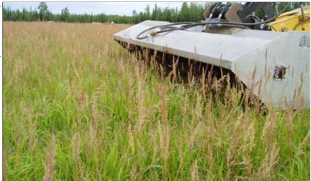
Using a seed stripper leaves the inflorescence (seed-head) intact, allowing for multiple equipment passes.
