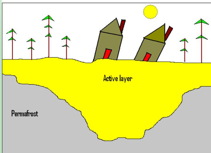
Thawing permafrost has expanded the active layer underneath these buildings. The removal of vegetative cover during construction allowed the soils to warm.
