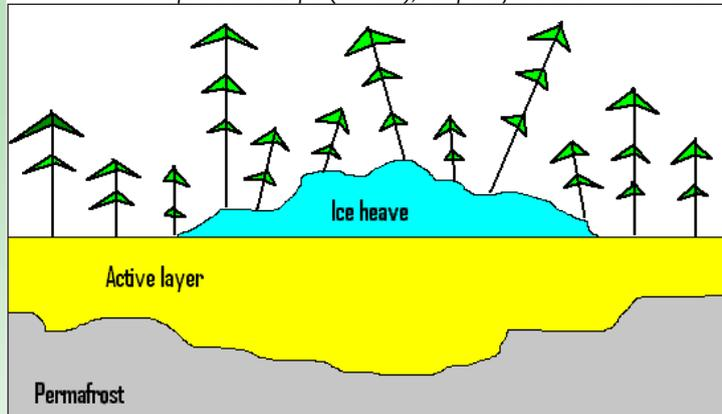
A "pingo" is created when water pooled in the active layer freezes, creating an ice heave above ground.
