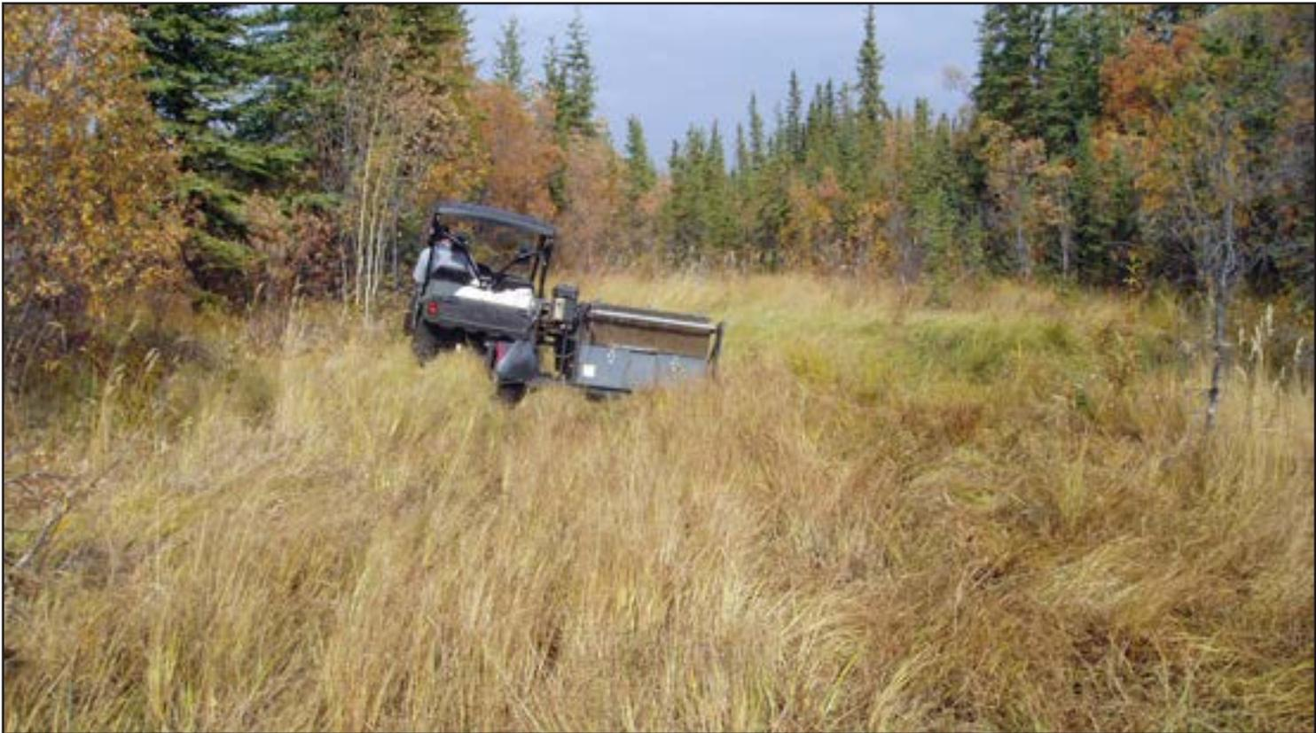
A pull-type seed stripper is an effective means of harvesting wild seed without damage to the surrounding environment.
