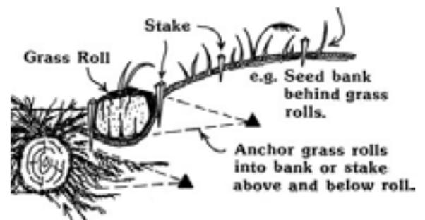
Sod clumps are also used in the restoration of erodible stream banks. Grass rolls use sod clumps wrapped in biodegradable fabric to stabilize river banks and quickly establish vegetation cover. For further explanation of this technique, refer to the ADF&G publication: 'Streambank Vegetation and Protection, a Guide for Alaska', or visit [www.adfg.alaska.gov/index.cfm?adfg=streambankprotection.main](http://www.adfg.alaska.gov/index.cfm?adfg=streambankprotection.main).
