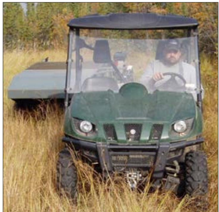
Mechanical seed stripper towed by an ATV
