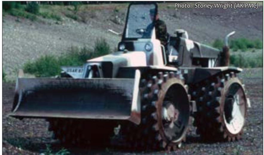
The wheels of this landfill compactor imprint the surface area, creating basins of micro relief in the seedbed
