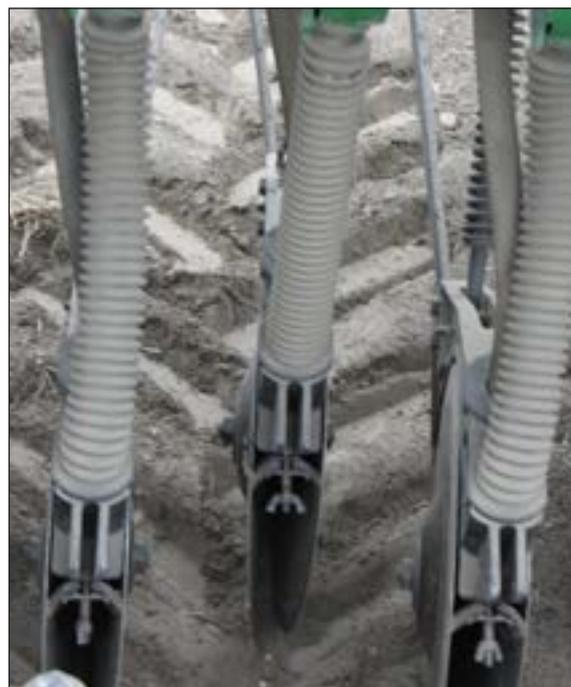
A drill seeder drops seed into a row prepared by the spinning discs.
