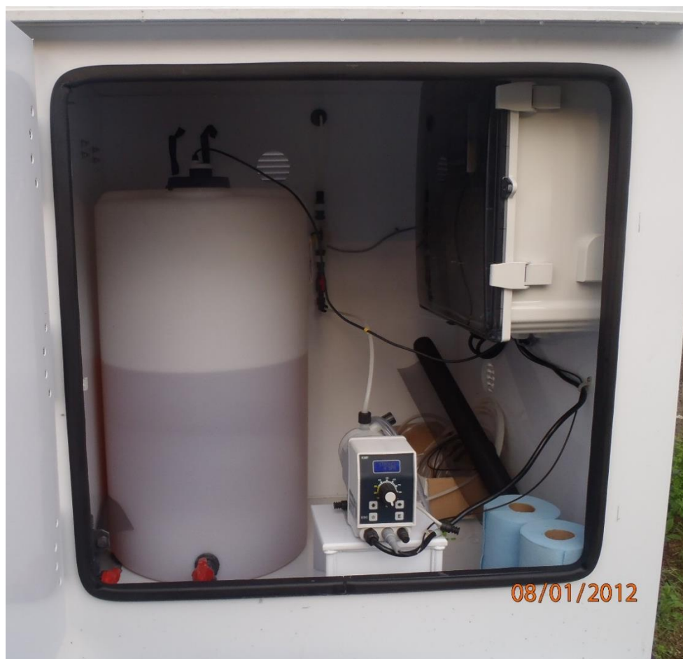
Fig. 8 Herbicide drip system apparatus for delivery of liquid herbicide (Sonar Genesis).
