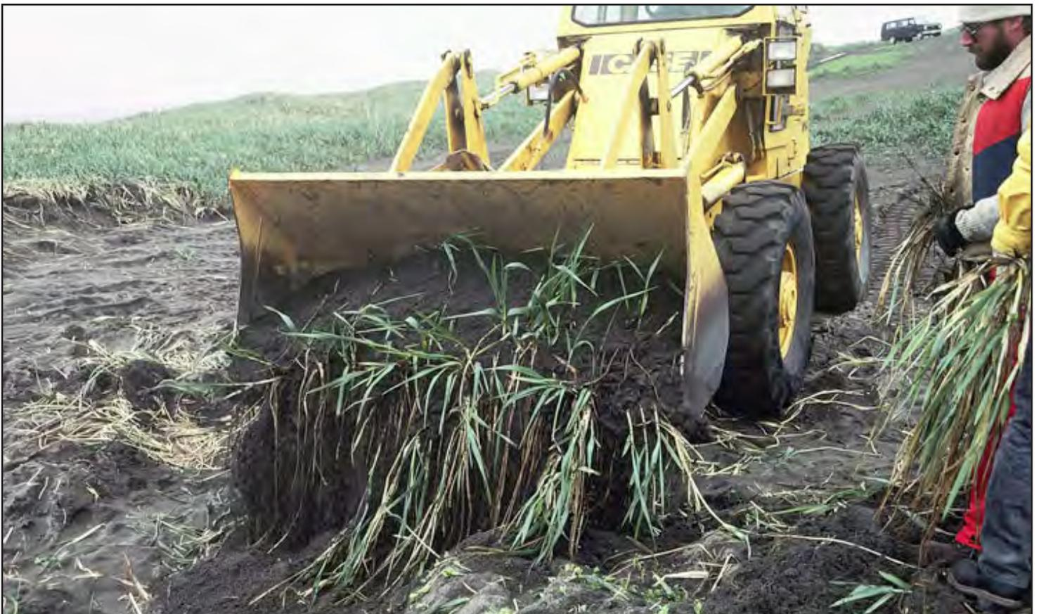
FIGURE a.10: Loader used to harvest sprigs
