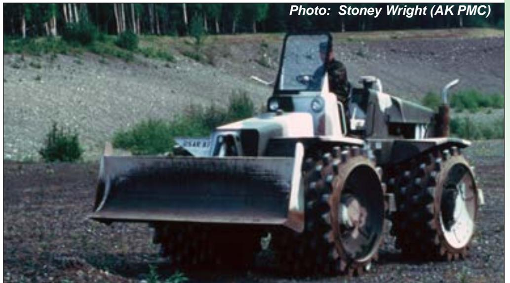
The wheels of this landfill compactor imprint the surface area, creating basins of micro relief in the seedbed
