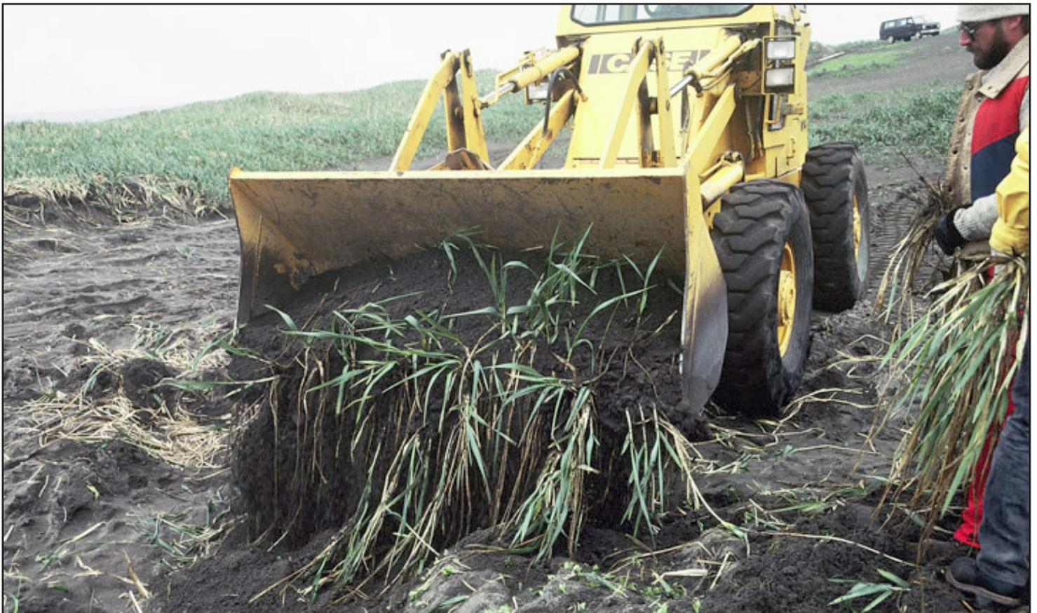
FIGURE a.9: Loader used to harvest sprigs
