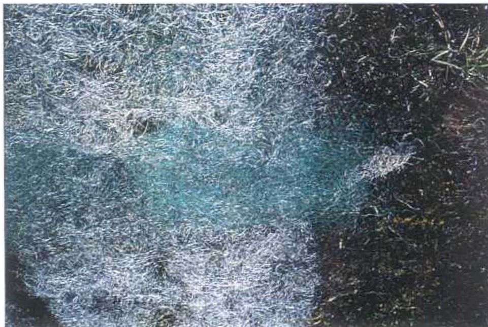
Figure 25. Loose Excelsior backing (netting) forming potential entrapment "nets".
