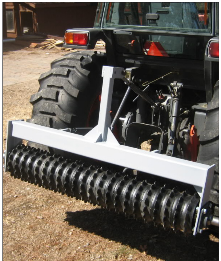
An imprinter can be used to firm sandy, silty or loose soils
